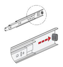
The rubber stops of type F dampen the impact of the slide in the two end positions. This feature minimizes noise development and increases the service life. Attached to the slides in a partially concealed, partially visible manner, the stops meet each of the requirements in regards to shape, material, and hardness.
