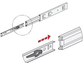
Type F has additionally a detach function through which the extension slides can be completely separated from one another in the area of the middle and inner slide. This feature not only facilitates mounting. It also allows the extension to be quickly removed, for example, when frequent maintenance work is performed on the components located behind.
