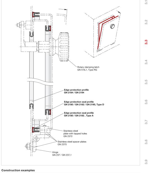
The construction depicted shows a standard application of edge protection profiles and edge protection seal profiles. The edge protection seal profiles are attached to the door and the fixed frame. The opening for the door is covered with an edge protection profile at its cut edge.
