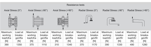
The maximum working loads are the loads which lead to a deformation of 2 mm of a single hinge.
