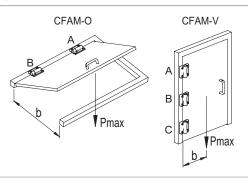
Hinges to be used for horizontal axis configuration (CFAM-O)
