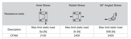
The max static load is the value above which the material may break thus prejudicing the hinge functionality. Obviously, a suitable factor, according to the importance and the safety level of the specific application must be applied to this value.
