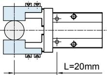
$$F \geq \frac{0.3 \times 9.8}{2 \times 0.1} \times 4 \geq 60(N)$$
