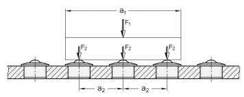
a<sub>1</sub> = shortest edge length of the load
