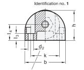
Bore for socket cap screw DIN 912
