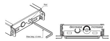
①Loosen the nut of adjustment screw.
