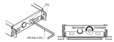
) Loosen the nut of adjustment screw.
