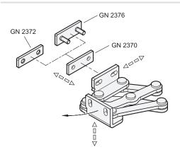
The Stainless Steel-Multiple-joint hinges can be adjusted in three planes during installation. For example, this allows tolerances to be adjusted or the required compressive forces for seals to be established. Two planes can be adjusted via the parallel or perpendicular slots in the fixing angle pieces. In the third plane, position corrections can be made using the Stainless Steel-Spacer plates GN 2370.
