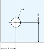
Boring position changes with the glass thickness.
