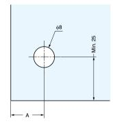
Boring position changes with the glass thickness.
