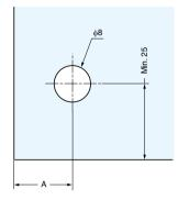
Boring position changes with the glass thickness.
