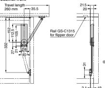
Left is the installation drawing when the travel length of rail GS-C1315-14 is 260mm. Installation position changes with the travel length of rail.
