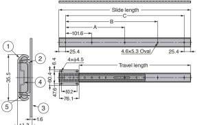
Inner member is located inside the retainer for precise movement.
