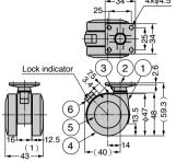
Drawing above shows the model with brake.
