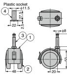
Drawing above shows the model with brake.
